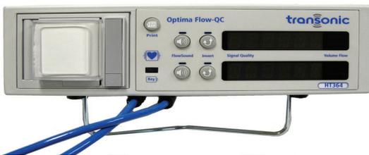
HT364 Dual-channel Optima®Flowmeter permits simultaneous measurements with two Flowprobes.
