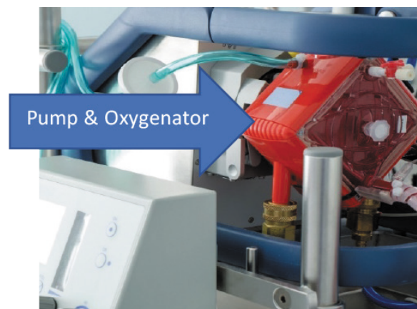
Cardiohelp System: combines oxygenator and pump into one device.
