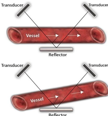
The ultrasonic beam intersects the vessel twice on its reflective path. With each intersection, the transit time through the vessel is modified by a vector component of flow. The full transit time of the ultrasonic beam senses the sum of these two vector components. With misalignment (bottom), one vector component of flow increases as the other decreases, with little consequence to their sum.
