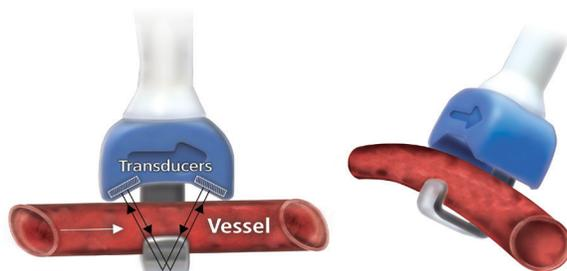
Schematic views of a Transonic® Perivascular Flowprobe. Using wide beam illumination, two transducers pass ultrasonic signals back and forth, alternately intersecting the flowing liquid in upstream and downstream directions. The Flowmeter derives an accurate measure of the “transit time” it takes for the wave of ultrasound to travel from one transducer to the other. The difference between the upstream and downstream integrated transit times is a measure of volume flow rather than velocity.
