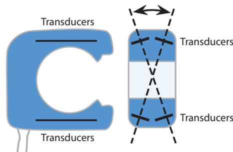
Confidence Flowprobes® use four transducers to create an X-beam ultrasonic illumination pattern to achieve a full vessel volume flow measurement.
