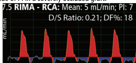
Figure 1: Stenotic flow waveform example in RIMA-RCA; flow is almost purely capacitive, with mostly antegrade flow in systole, mostly retrograde flow in diastole, and very low mean flow rate. As a result PI is high.
