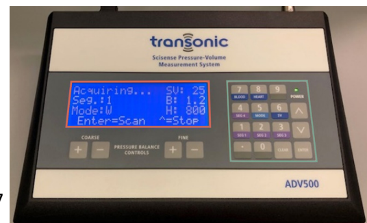
Fig 5: Highlighted in red is the main data collection screen while green highlights the quick access buttons on the keypad
