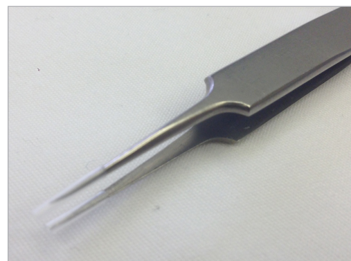
Place polyethylene tubing over the forceps' tips to protect the catheter body from damage.
