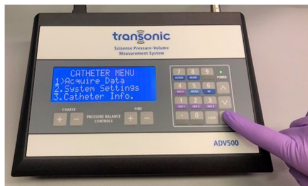
Fig. 2: Selecting "Acquire Data" from the catheter menu turns the catheter on.
