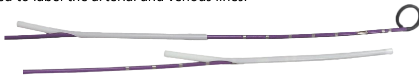
Fig. 4: 5F PV Catheter with straightening introducer retracted (top) and engaged (bottom) to uncurl pigtail.
