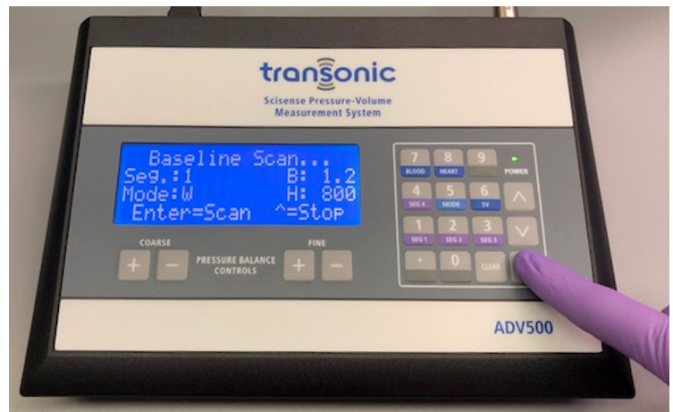
Fig. 4: A baseline scan is performed by pressing "Enter" during data collection. This process allows for volume to be calculated accurately.
