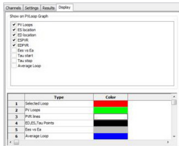
Display tab for selecting the parameters visible on the graph and their colors.
