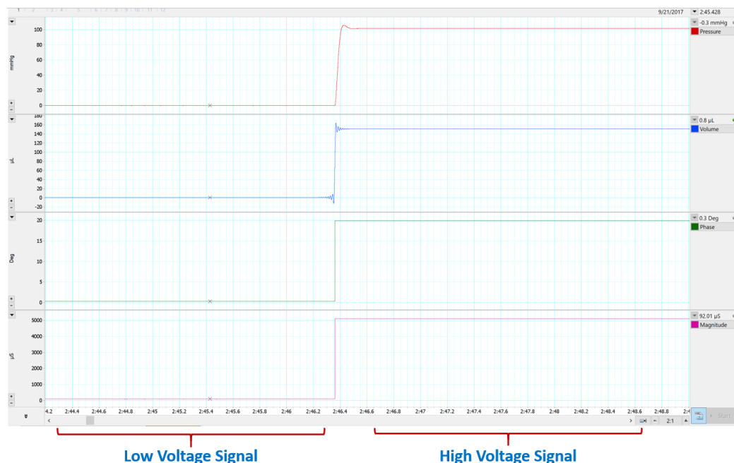
Fig. 8: Left flat line represents the low voltage signal coming from the ADV500 while the right flat line represents the high voltage signal. These will be used for unit conversion in the software.
