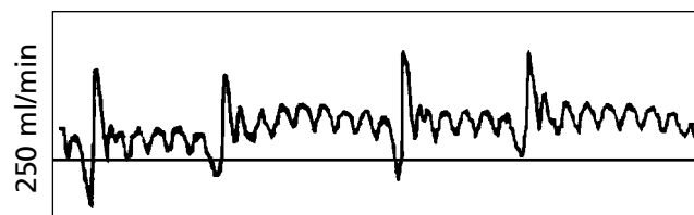
Fig. 1: Instantaneous flow ranged from 200 to 350 ml/min. This pulsatile flow example is from an acute experiment in an anesthetized dog. Note the periodic spikes from respiratory activity. Typical mean flow from chronic experiments ranged from 376 to 450 ml/min.
