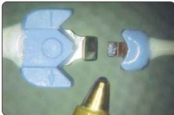
Fig. 2: New 0.5PSB (right) with standard 0.5 mm V probe (left) and ballpoint pen tip (bottom).
