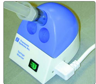
Syringe filled with saline inserted into the Transonic Syringe Warmer for Cardiac Output measurements with Transonic Flow-QC Hemodialysis Monitors.
