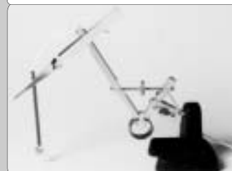
Handles on V-probes allow for stable position with a micromanipulator.
