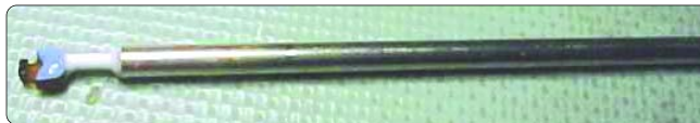
Bottom: Nanoprobe with handle for acute blood flow mapping in the mouse.
