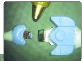
Top: New 0.5PSB (left) with standard 0.5 mm V probe (right) and ballpoint pen tip. Middle: 1.5PSL probe for ascending aortic blood flow as shown in trace on left.
