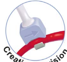
Fig. 1.1: Intraoperative perivascular flowprobe measures direct volume flow during AV access creation or revision surgeries.
