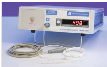
Fig 3.4: HVT100 Endovascular Flowmeter measures intragraft blood flow in the arteriovenous (AV) vascular access to provide quantitative information about access functionality during angioplasty.
