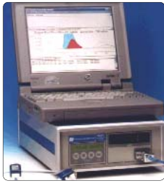
HD01 Monitor with laptop computer and H4D sensors
